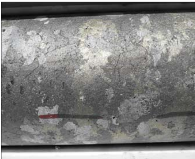
Mutooroo drillcore showing massive sulphide ore with abundant copper sulphide in the form of chalcopyrite (brassy yellow mineral), plus pyrrhotite (bronze mineral) and barren quartz (white) from approx. 92 metres depth
