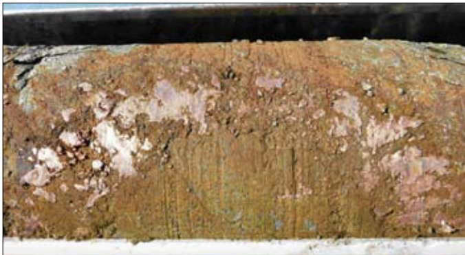
Kalkaroo drill core from approx. 110 metres depth with rich native copper metal distributed through the weathered host formation
