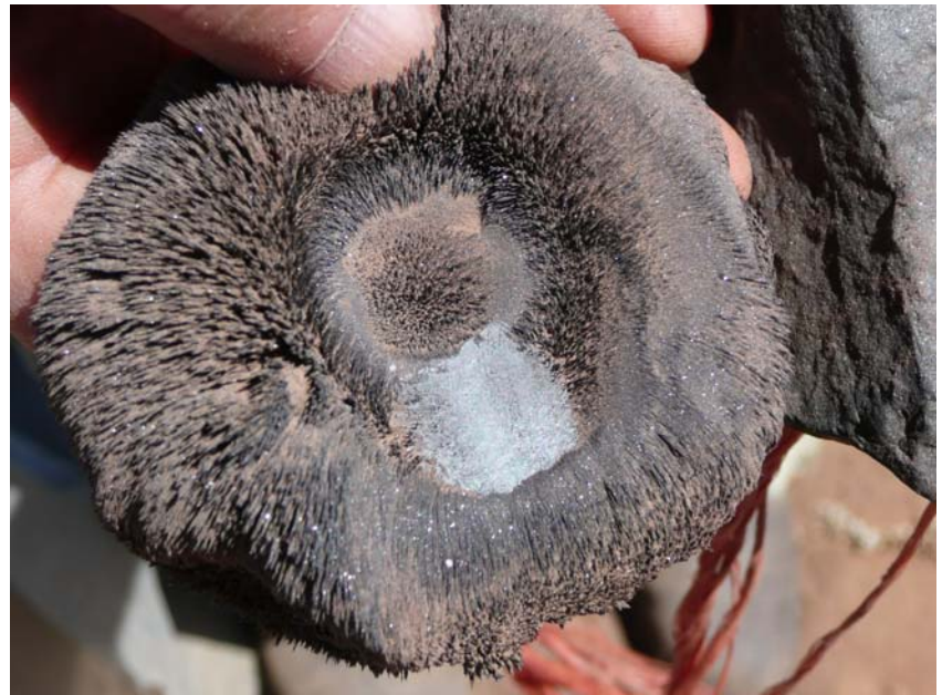
Coarse-grained magnetite recovered from drill sample by a hand magnet
